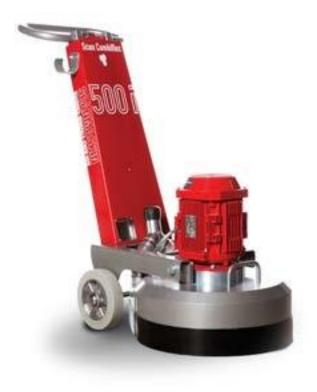
The Scan Combiflex 500i is a highly effective and powerful grinder despite its compact size. This single speed planetary machine is very reliable and simple to use. It is robust and works well for surface preparation work, such as rough grinding and coating removal.
